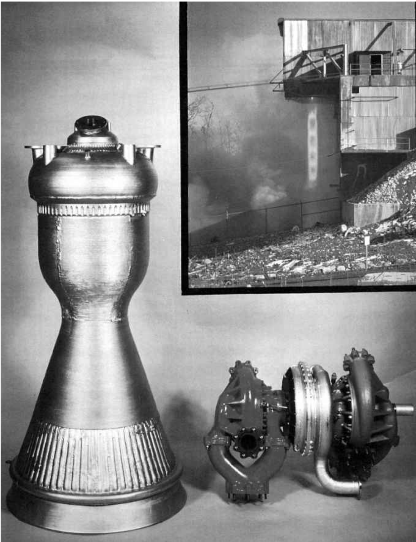
The Reaction Motors XLR30-RM-2 liquid-propellant rocket engine was the leading candidate for the X-15 powerplant. The XLR30 had been developed from the XLR10 that powered the Viking sounding rocket developed for the Naval Research Laboratory. Twelve Vikings were launched
