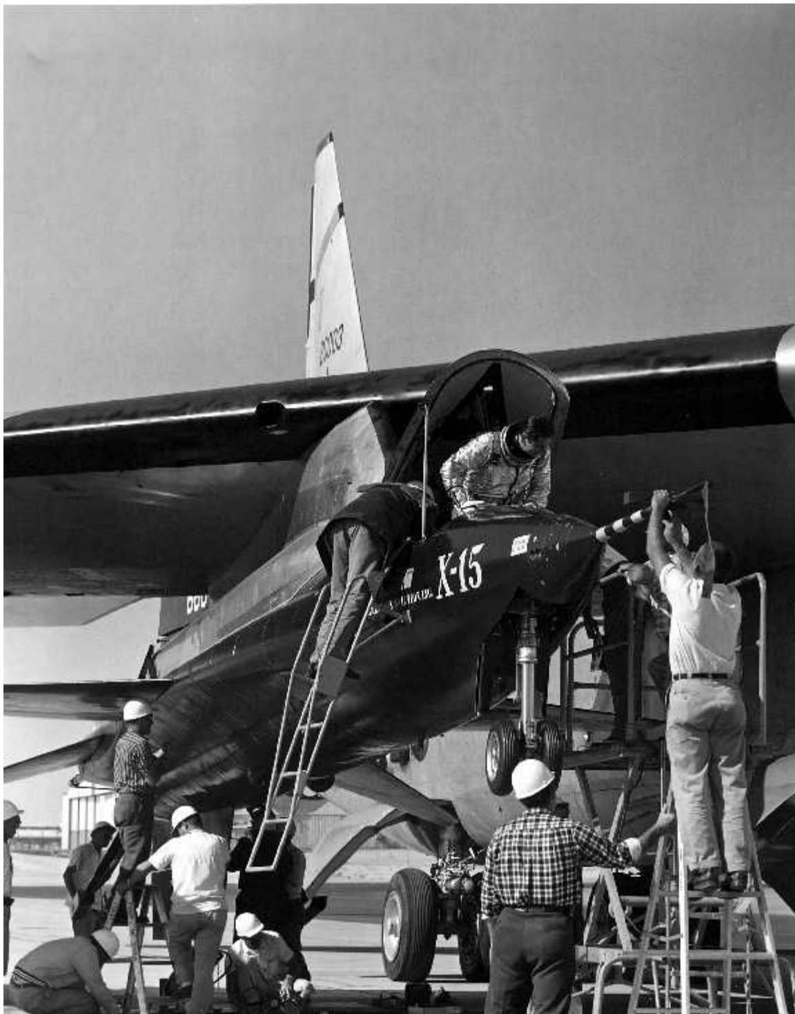
Scott Crossfield climbs out of X-15-1 after the first captive-carry flight. The X-15 landing gear had been deployed during the flight to demonstrate it would work after being cold-soaked at altitude. A member of the ground crew installs protective covers on the nose-mounted air data boom. (AFFTC History Office)
