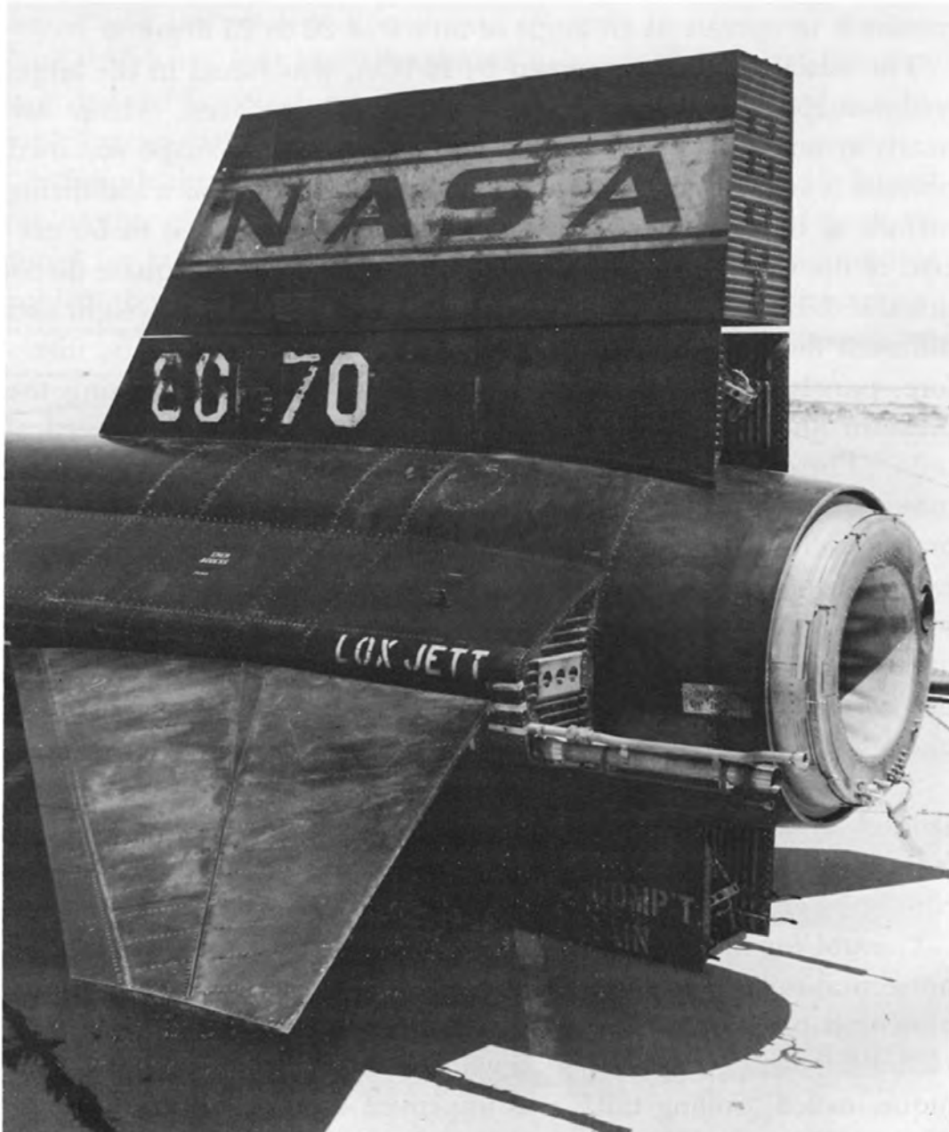
The blunt aft ends of the X-15's side fairings, vertical tails, and the rocket-engine nozzle represent one of the many compromises that a hypersonic configuration demanded. Together they produce as much drag as an F-104 jet fighter.
