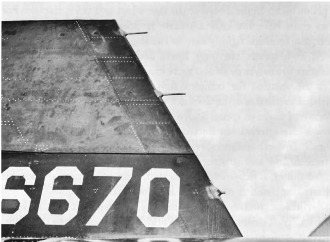
Pressure tubes in the leading edge of the X-15's upper vertical tail measure airflow conditions in the wake of the fuselage. The craft's instrumentation, elaborate despite weight and volume restrictions, measured pressure at 160 locations.
