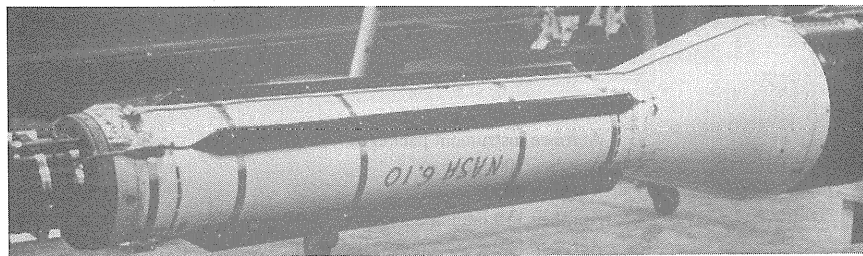
Figure 32c - Aerobee 300A, third stage motor with DOVAP transducers and antennas.
